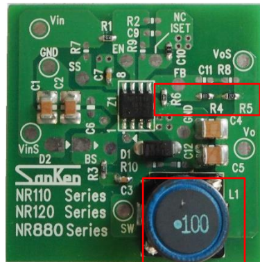
Figure 8-2. Output Voltage Adjustment Resistors and Inductor
