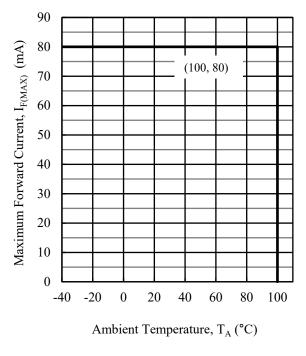
Figure 1. I<sub>F(MAX)</sub> vs. T<sub>A</sub>
