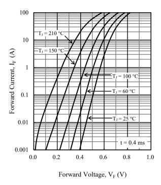
Figure 3. I<sub>F</sub> vs. V<sub>F</sub> Typical Characteristics
