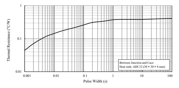
Figure 6. Typical Transient Thermal Resistance (2)
