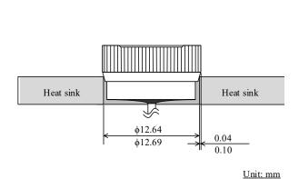
Figure 7 Recommended Hole Size and Interference
