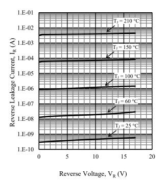
Figure 4. I<sub>R</sub> vs. V<sub>R</sub> Typical Characteristics
