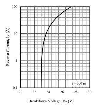
Figure 5. Iz vs. Vz Typical Characteristics
