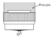
Figure 9 Recommended Press Pin Form
